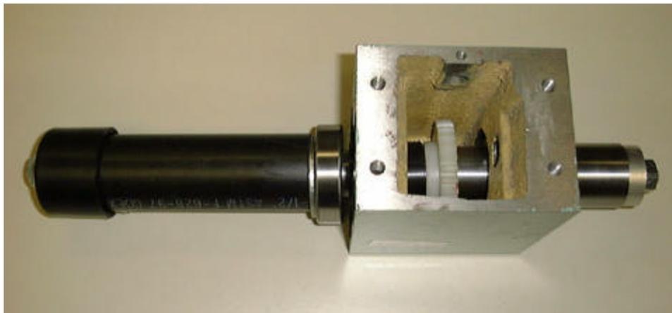
7. Tighten the nuts to press the spindle into the spindle box. Tighten until the bottom bearing is seated in the housing.
