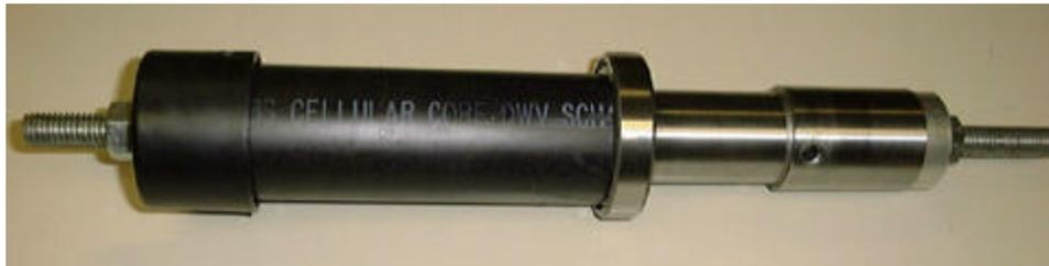
3. Tighten the nuts to press the bearing into place. Be sure it is seated against the step on the spindle.
